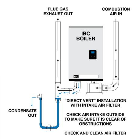
Figure 13: Direct vent - intake, exhaust and condensate removal system with optional air intake filter (filtration may also be used on indoor air applications as required)
