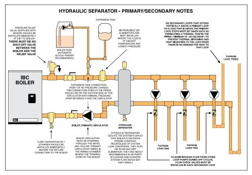
Figure 25: Important Primary/Secondary piping details with hydraulic separator
