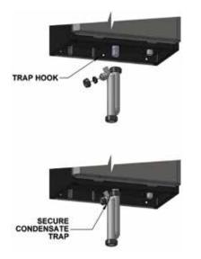
Figure 17: Condensate trap installation
