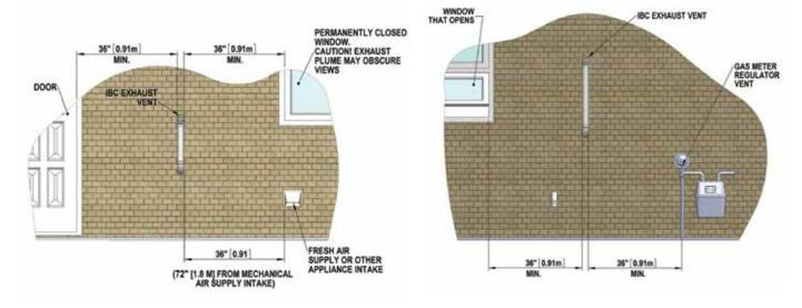
Figure 8: Vent terminal clearances
