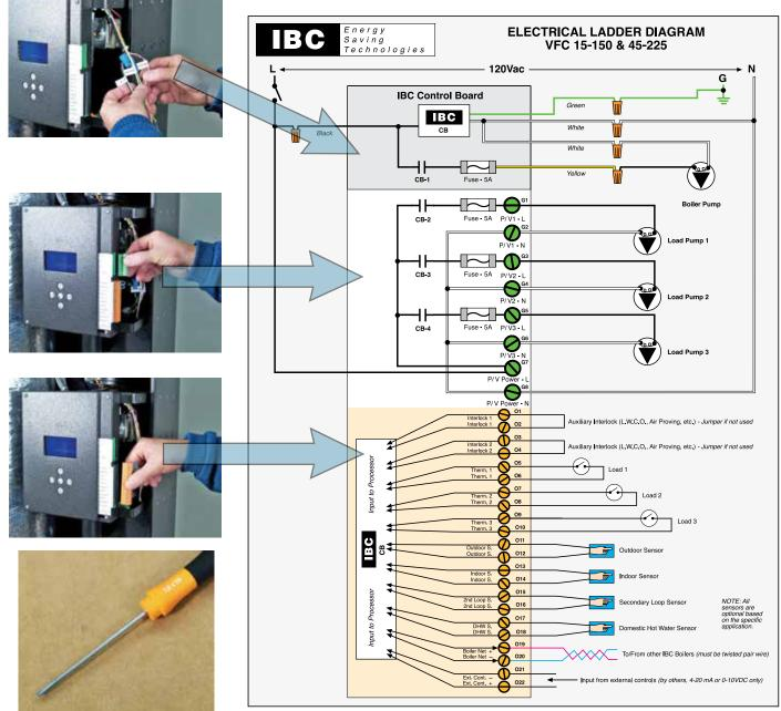
A 2.5 mm Slot screwdriver is required for the bottom terminal strip. Broader or narrower blades may damage the terminal screws.
