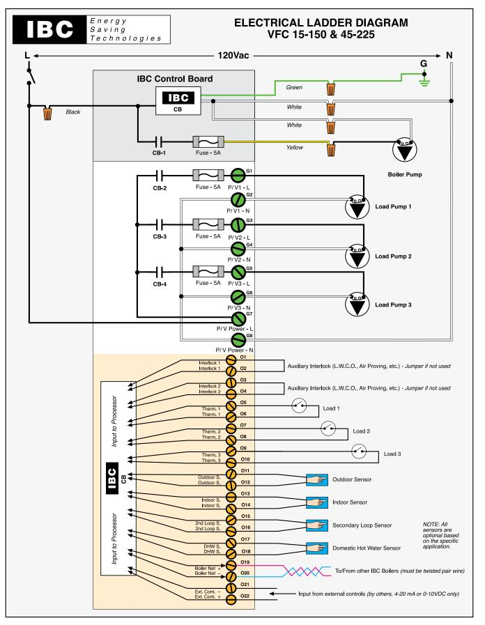
Diagram 6.2-2: Ladder wiring diagram
