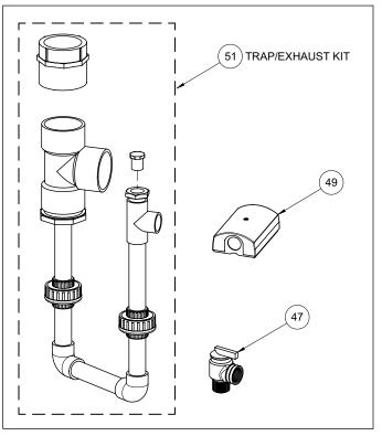
Diagram 6.1-4: Accessory parts kit (shipped with boiler)
