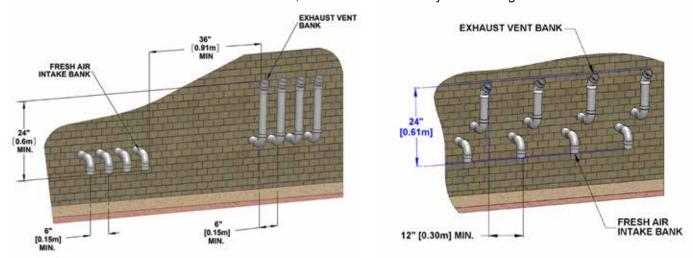
Figure 5: Sidewall vent termination - multiple vent piping configuration
