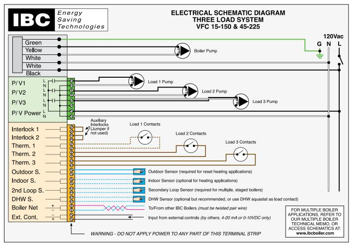
Diagram 6.2-1: Pictorial wiring diagram
