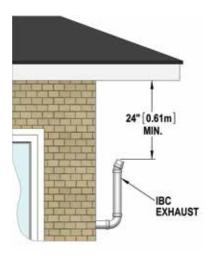
Figure 6: Vent terminal clearances
