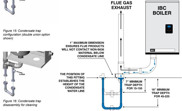
Figure 14: Condensate trap configuration (single union option shown)
