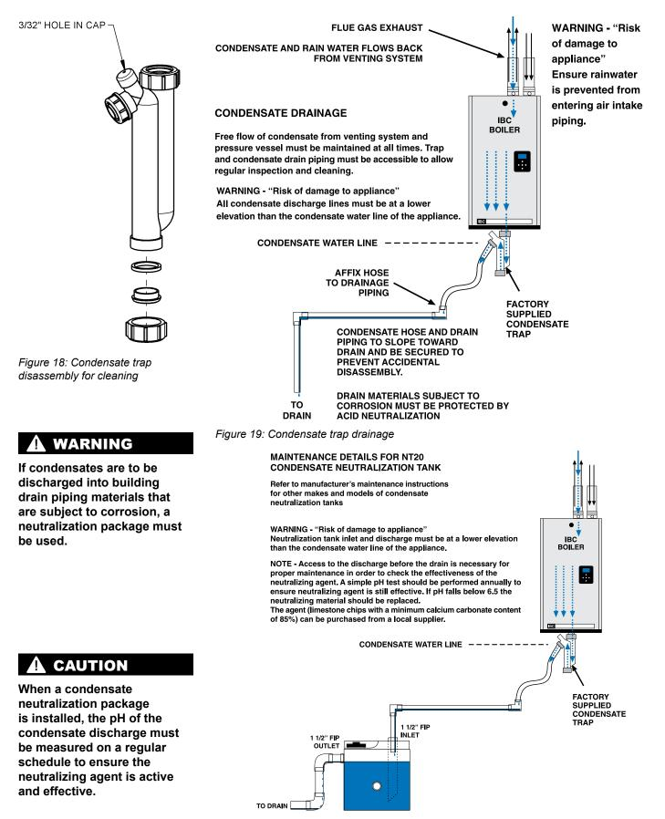
Figure 20: Condensate neutralization tank
