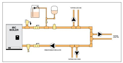
Figure 22: Basic Primary/Secondary piping concept
