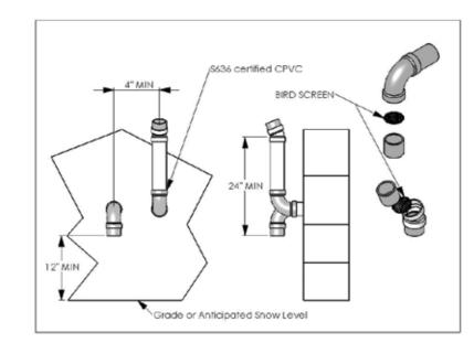
Figure 4: Sidewall vent termination - piping configuration
