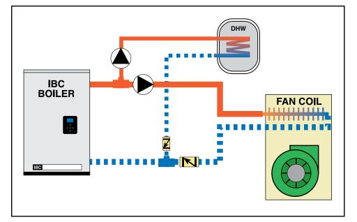
Figure 27: Two pump, two load - parallel piping concept
