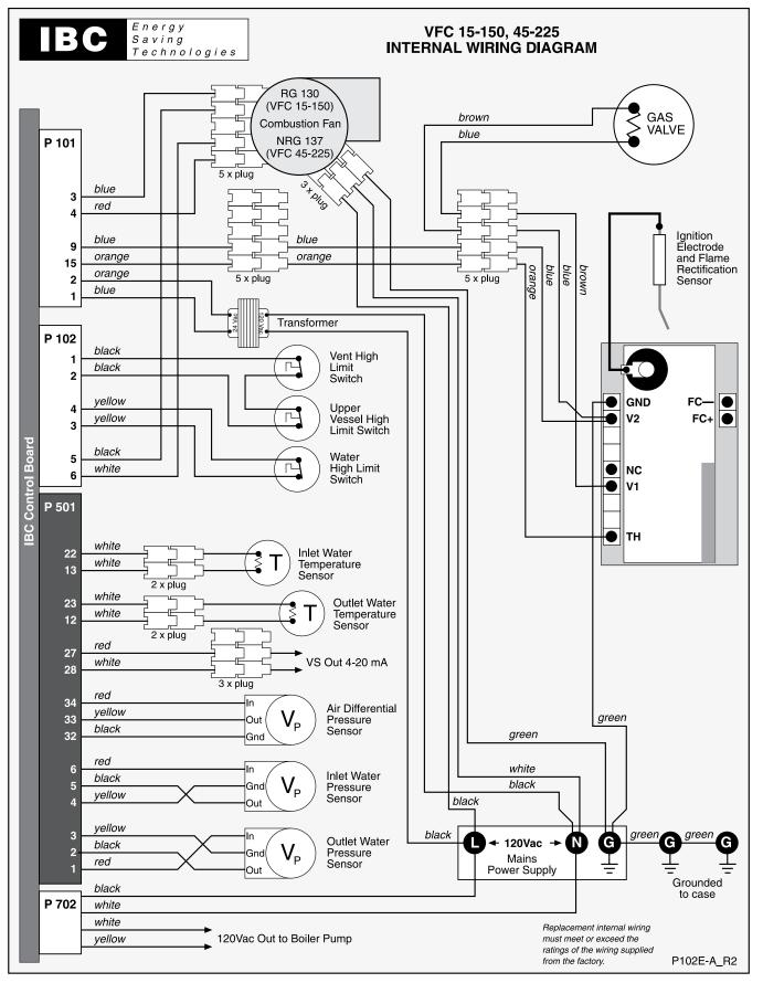
Diagram 6.2-3: Internal wiring diagram
