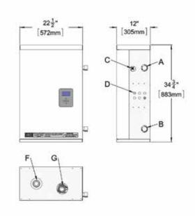
Figure 1a: Dimensions / Connections for VFC 15-150
