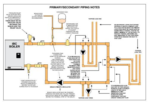
Figure 23: Important Primary/Secondary piping details
