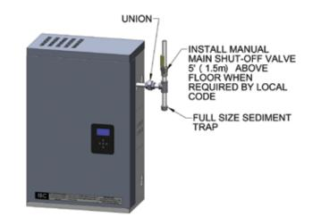
Figure 28: Typical gas piping
