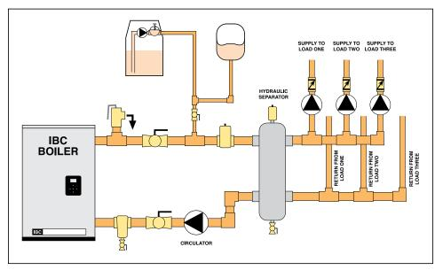
Figure 24: Primary/Secondary piping concept with hydraulic separator
