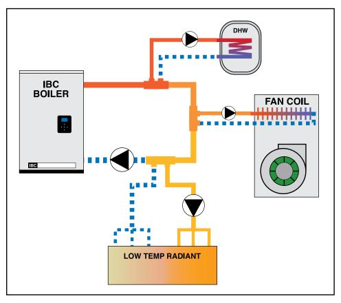
Figure 26: Basic Primary/Secondary, 3 load piping concept
