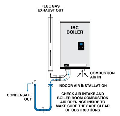
Figure 11: Indoor air - intake, exhaust and condensate removal system
