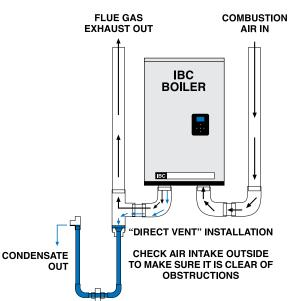
Figure 10: Direct vent - intake, exhaust and condensate removal system
