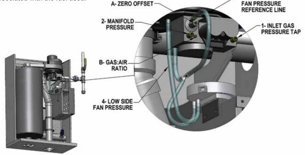
Figure 31: Gas Valve and Pressure Reference System
