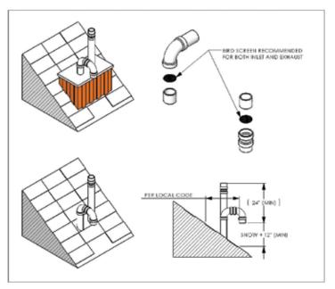
Figure 3: Rooftop vent terminal configurations
